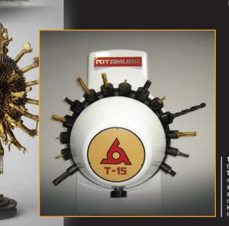
1971 – Kitamura succeeds in developing the first fully automated T-12 Vertical Machining Center I-12 Vertical Machining Center with an ultra-fast (2 second) 12 station automatic tool changer – The fastest in the world at the time. With the ATC design based on the Senju-Kannon statue, a muti-tasking deity, Kitamura began mass production for sale Worldwide.
