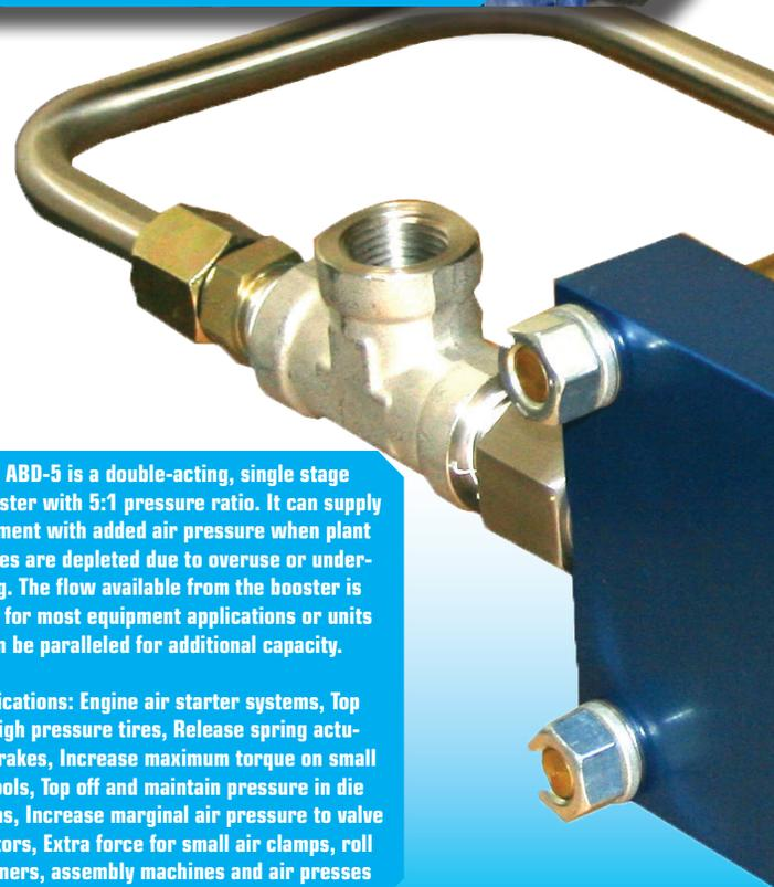
The ABD-5 is a double-acting, single stage air booster with 5:1 pressure ratio. It can supply equipment with added air pressure when plant supplies are depleted due to overuse or undersizing. The flow available from the booster is ample for most equipment applications or units can be paralleled for additional capacity.
