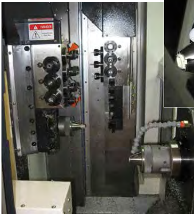
The turning center has two opposing spindles and two gang turrets. The production parts are so small that custom collets are needed to permit access to all of the machined features. The custom collets were supplied by Hardinge.
