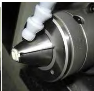
The turning center has two opposing spindles and two gang turrets. The production parts are so small that custom collets are needed to permit access to all of the machined features. The custom collets were supplied by Hardinge.
