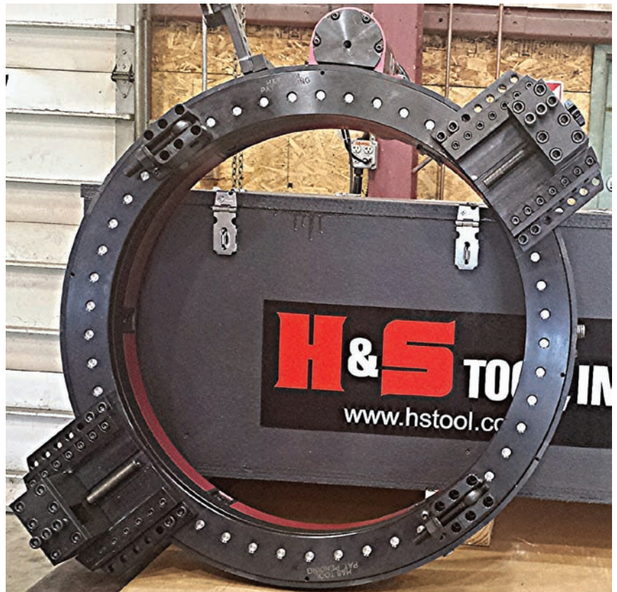
A completed clam cutter. Wagner Machinery manufactures 80% of the component parts which are sent to H & S Tool, Inc. for assembly.
