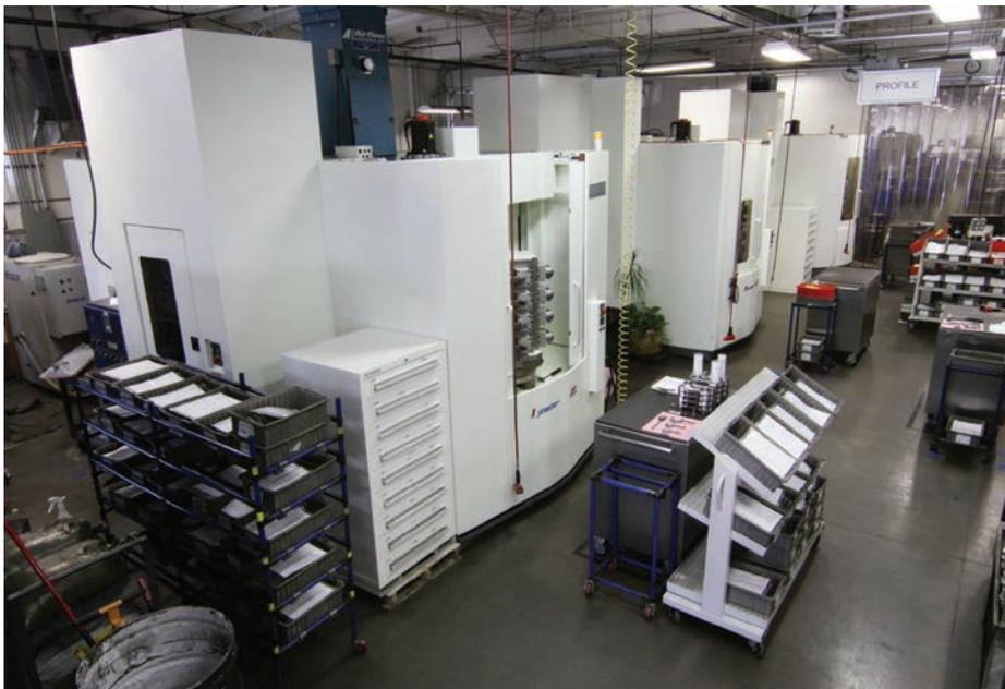
Optimized workflow in the Kitamura aisle of the Profile Machining Department at CP-Carrillo. CP-Carrillo has two Mycenter-HX400IFTGA (400 mm) and three Mycenter-HX500iTGA (500 mm) horizontals.
